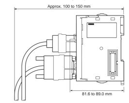
Note: Consider the following points when expanding the configuration: The total length of I/O Connecting Cable must not exceed 12 m. I/O Connecting Cables require the bending radius indicated below.
