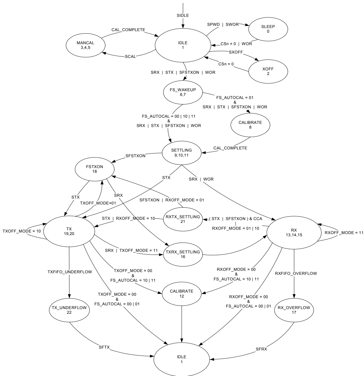
Figure 16: Complete Radio Control State Diagram
