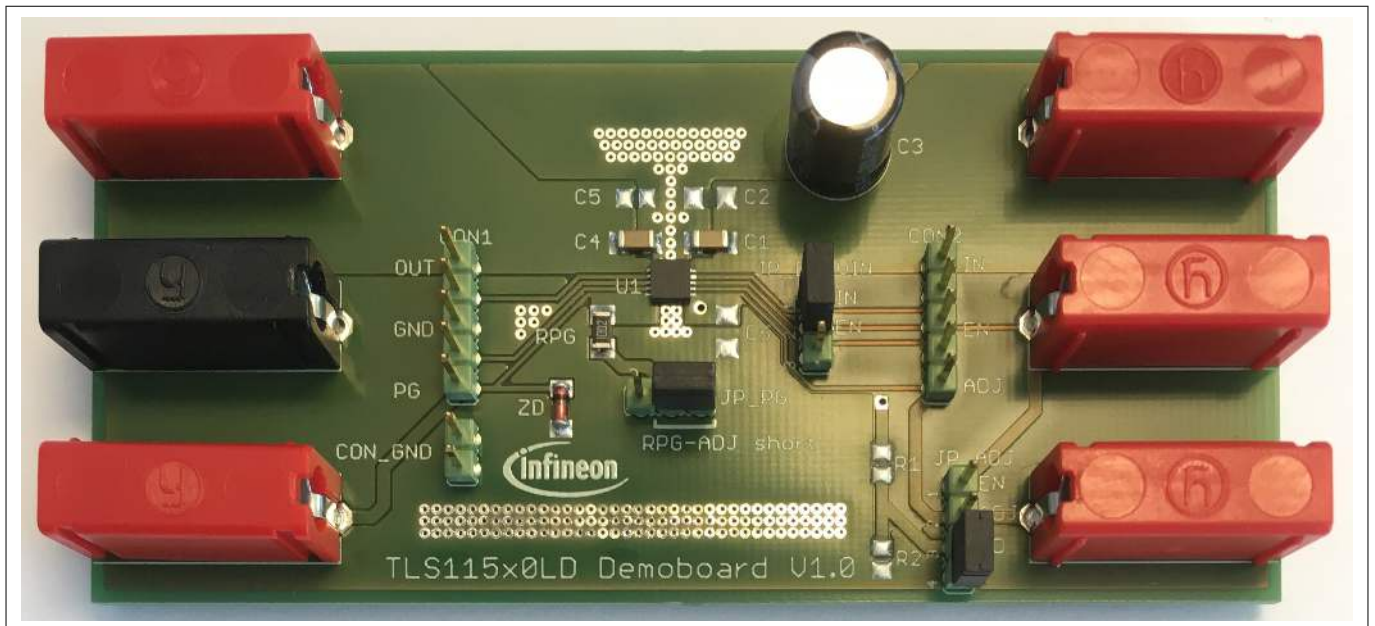
Figure 3 OPTIREG™ linear voltage regulator TLS115x0LD demoboard
