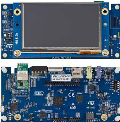
STM32H7B3I-DK board top and bottom views. Fanout board not shown. Pictures are not contractual.
