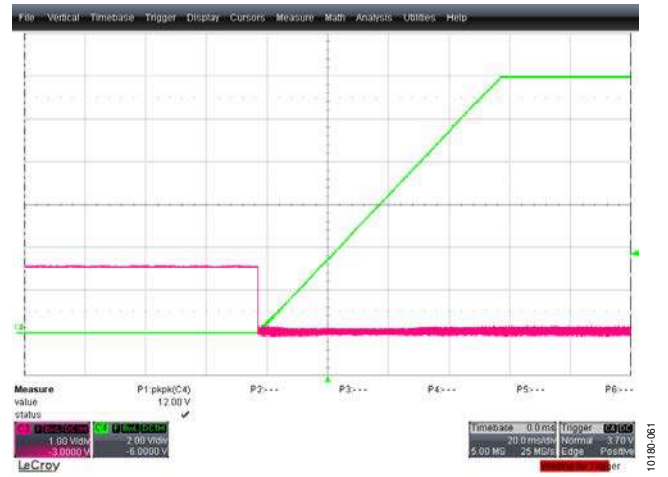
Figure 62. OrFET Turn-On Green Trace: Output Voltage, 2 V/div, 20 ms/div Red Trace: GATE Signal Voltage, 2 V/div, 20 ms/div
