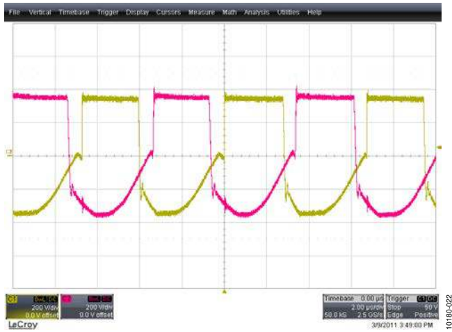
Figure 23. Transformer Primary Waveform at 25 A Load, 350 V DC Red Trace: Voltage Across T1 Primary (Phase 1), 200 V/div, 2 µs/div Yellow Trace: Voltage Across T2 (Phase 2), 200 V/div, 2 µs/div
