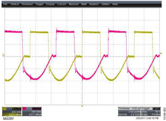
Figure 24. Transformer Primary Waveform at 25 A Load, 400 V DC Red Trace: Voltage Across T1 Primary (Phase 1), 200 V/div, 2 µs/div Yellow Trace: Voltage Across T2 (Phase 2), 200 V/div, 2 µs/div
