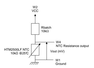
$$V_{OUT}(mV) = \frac{Vcc(mV) * NTC_{HTM 2500LF}(\Omega)}{R_{batch}(\Omega) + NTC_{HTM 2500LF}(\Omega)}$$
