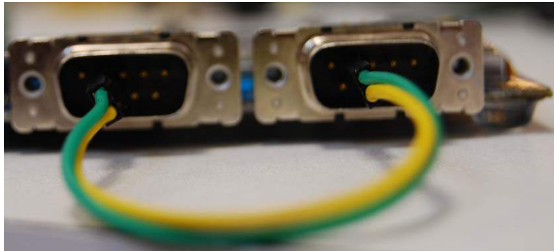
Figure 2-3. CAN loopback on the AT32UC3C-EK
