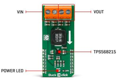
The onboard voltage divider connected to the MODE pin of the IC is used to set the device to work with the fixed PWM frequency of 800kHz, DCM/Eco-mode<sup>™</sup> for light loads, and to set the limiting current to about 7A.
