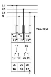
$3(N)\sim230$  V/132 V measuring range with connected neutral conductor, 230 V AC supply voltage
