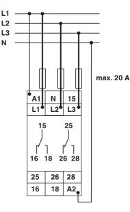
3(N) ~ 230 V/132 V measuring range, 24 V AC supply voltage 3(N) ~ 230 V/132 V measuring range, 230 V AC supply voltage
