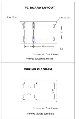
Dimensions in mm. Tolerance:  $\pm$  .25 mm
