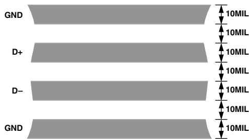
Figure 8. Arrangement of Signal Tracks
