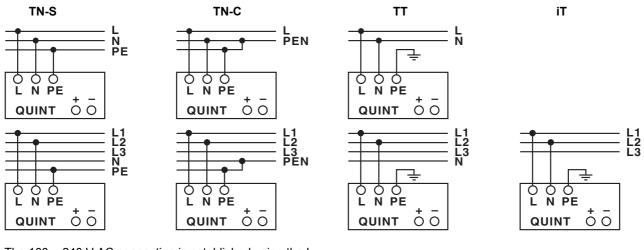
The 100-...240 V AC connection is established using the L, N and PE screw connections.
