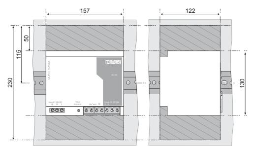
Slim-style installation: Installation depth 125 mm (+ DIN rail)
