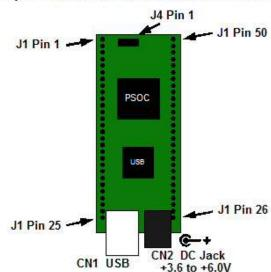
Top View (J1 Interface Headers on Bottom of PCB)
