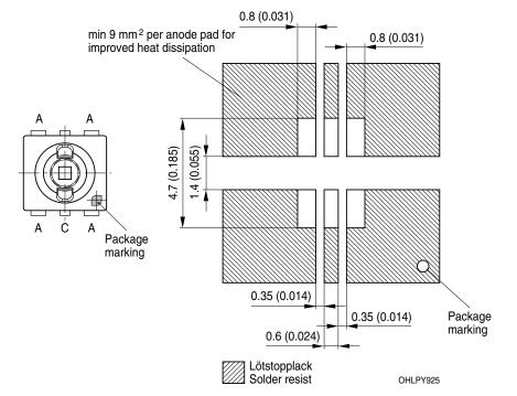
For superior solder joint connectivity results we recommend soldering under standard nitrogen atmosphere. Package not suitable for ultra sonic cleaning.
