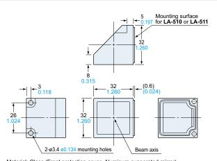
Material: Glass (Front protection cover, Aluminum evaporated mirror) Polyetherimide (Enclosure)
