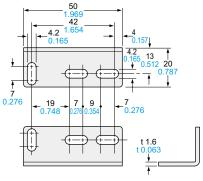
Material: Cold rolled carbon steel (SPCC) (Uni-chrome plated)
