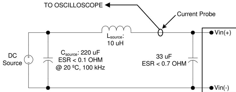
Note: Measure input reflected-ripple current with a simulated source inductance ( $L_{test}$ ) of 10 uH. Capacitor  $C_s$  offsets possible source impedance.
