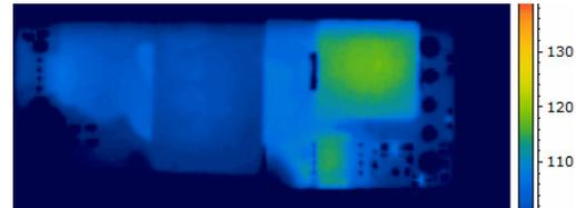
Thermal Image of module @ 48Vin, 200LFM & 70C
