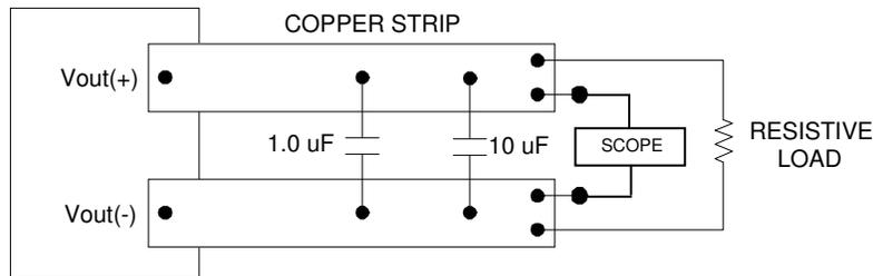
Note: Use a 1µF X7R ceramic capacitor and a 10µF tantalum capacitor. Scope measurement should be made using a BNC socket. Position the load 3 in. [76mm] from module.
