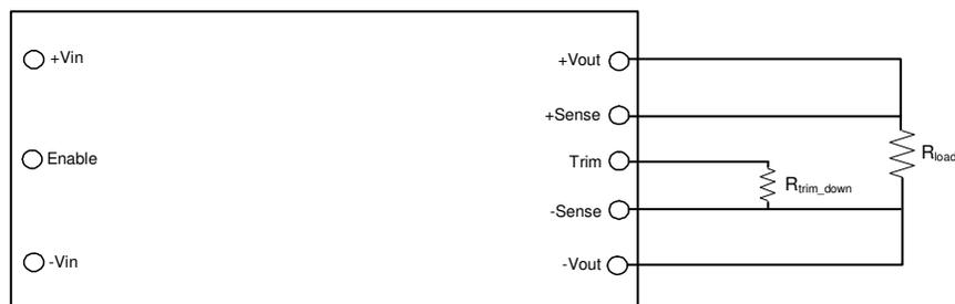
Figure 16. Trim DOWN circuit configuration
