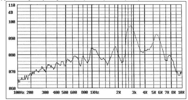
Typical Frequency Response (3 V0-p sine-sweep with microphone spaced at 10cm)
