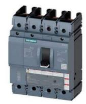
circuit breaker 3VA5 UL frame 250 breaking capacity class H 65kA @ 480V 4-pole, line protection TM230, FTAM, In=90A overload protection Ir=90A fixed short-circuit protection Ii=5...10 x In N conductor protection 100% without connection
