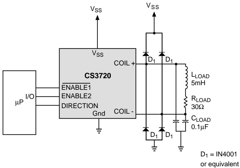
Note: A heatsink is required for 2A operation.
