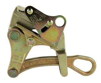
This lightweight, compact grip pulls ACSR cable from 0.16 to 0.90-Inch (2.3 to 0.4 CM) in diameter. The round jaw provides maximum contact with the cable while minimizing deformation. The hot latch closes automatically to guard against the grip accidentally disengaging from wire.
