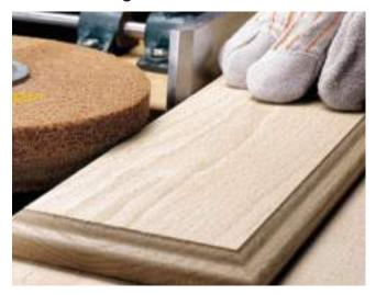
This wheel is a custom designed non-woven abrasive product for use on white wood sanding. An advantage of this wheel is the open construction and the use of garnet mineral, reducing the potential for part burning. The Scotch-Brite™ Woodworking Wheel may be used in its straight form or shaped to various profiles.
