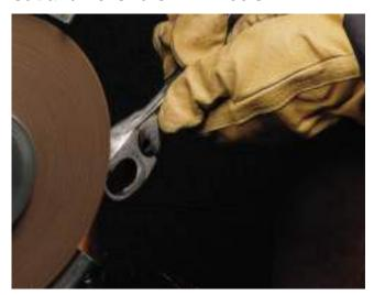
Cut and Polish / CPM Wheels are heavy duty wheels for more aggressive blending and finishing. These long lasting wheels perform well on tough blending and finishing applications such as removing surface defects, coarse grindlines, blending forging marks and machining mismatches while leaving a uniform grain finish.
