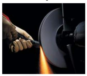
The 3M™ XR Metalworking Wheel is loaded with mineral and is designed for demanding applications such as removing sharp burrs that may drastically reduce the life of a non-woven abrasive or rubber bonded wheel.
