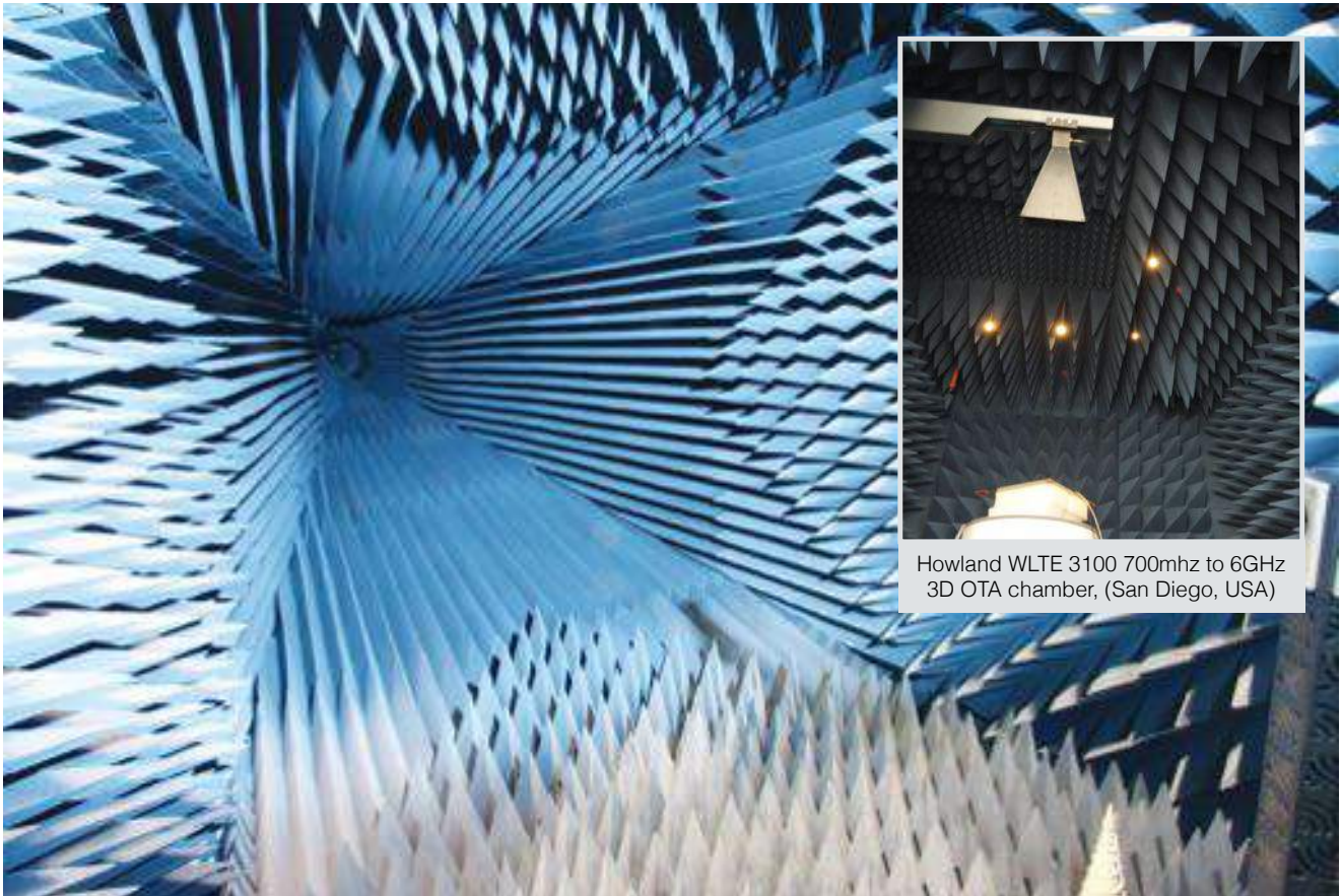
Taoglas' 12 metre 400 MHz to 6000 MHz ETS Lindgren 3D Tapered Anechoic Chamber in Wexford, Ireland
