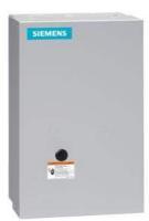
Non-reversing NEMA contactor, Size 4, Three phase full voltage, Contactor amp rating 135A, 3 wire (NO aux included), 208VAC 60Hz coil, Non-combination type, Enclosure NEMA type 1, Indoor general purpose use, Standard width enclosure
