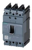
circuit breaker 3VA5 UL frame 125 breaking capacity class H 65kA @ 480V 3-pole, line protection TM210, FTFM, In=15A overload protection Ir=15A fixed short-circuit protection Ii=20 x In UL 489 SB (naval), 50° C without connection
