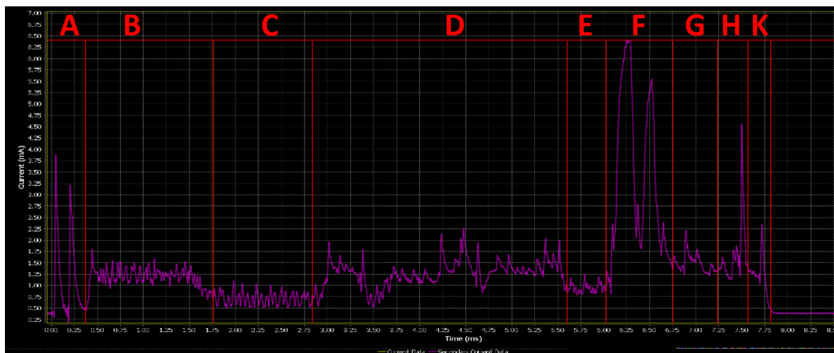
Figure 129: BLE Connection power profile
