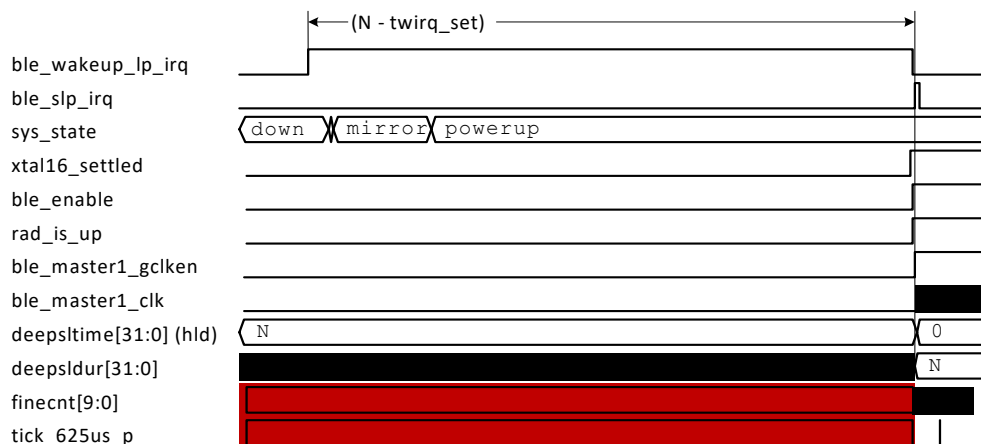
Figure 125: Exit BLE Deep Sleep Mode at predetermined time (zoom out)
