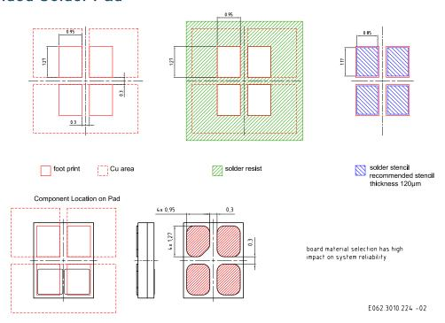
For superior solder joint connectivity results we recommend soldering under standard nitrogen atmosphere. Package not suitable for ultra sonic cleaning. To ensure a high solder joint reliability and to minimize the risk of solder joint cracks, the customer is responsible to evaluate the combination of PCB board and solder paste material for his application.
