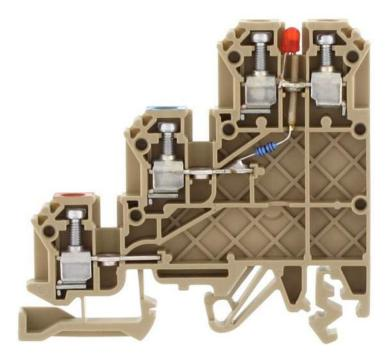
Three-level initiator terminal, Screw connection, Mounting type:Mounting rail TS 35/7.5 and TS 32, Rated cross-section: 2.5 mm<sup>2</sup>, Width: 5 mm, Colour: Beige
