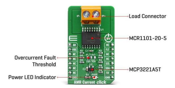
VOC pin is connected directly to VOC (Reset) pin on mikroBUS™. Voltage on this pin defines the overcurrent detection OCD threshold level. Briefly driving this pin to VCC resets and rearms OCD circuit.
