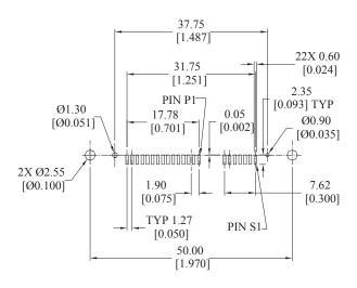
RECOMMENDED PCB LAYOUT TOLERANCE:  $\pm 0.05 [0.002]$
