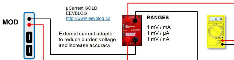
Figure 9: Using an external precision current adapter to minimize burden voltage effects in low current measurements.
