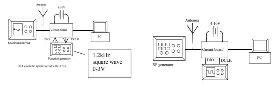
The above figures show typical evaluation connections for TX (left) and RX (right). Optimal settings for achieving the best possible sensitivity are available for download from the Chipcon web site. Chipcon recommends that these settings be used when maximum range is paramount. For details on how to use the SmartRF® Studio software please refer to the SmartRF® Studio User Manual.
