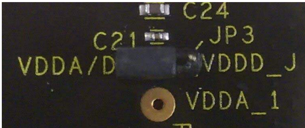
Figure 2. Selecting the VDDA/D side will select power source from on-board regulators powered by USB; Selecting the VDDD_J side will select external bench power supply
