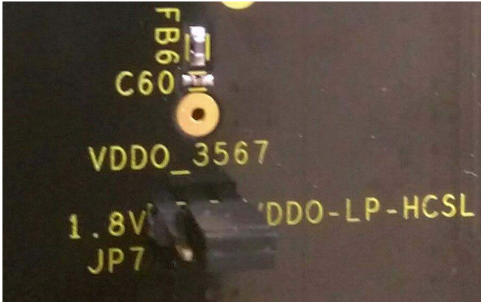
Figure 4. In the 3-way header, the middle pin is the output node and the 1.8V and VDDO_LP_HCSL on either side. Jumper settings are selected according to the output voltage required for outputs 3, 5, 6 and 7.
