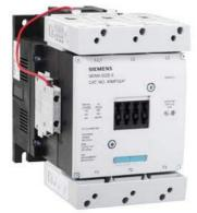
Vacuum NEMA contactor, Size 6, Three phase full voltage, Contactor amp rating 540A, 3 wire (NO aux included), 110-127V 50-60Hz/DC coil, Non-combination type, Enclosure NEMA type (open), No enclosure
