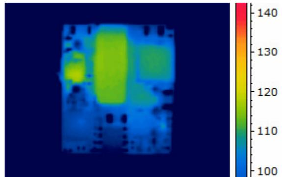
Figure 6. Thermal Image of CPZ4A36 4A output, 70C Ambient, 200lfm airflow, Vin = 48V, T<sub>max</sub> = 118°C
