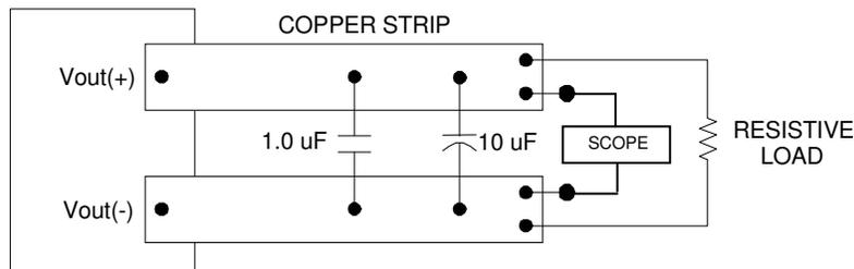
Use a 1.0 $\mu$ F X7R ceramic capacitor and 10 $\mu$ F @20V low ESR tantalum capacitor. Scope measurement made using a BNC socket. Position the load 3 in. [76mm] from module.
