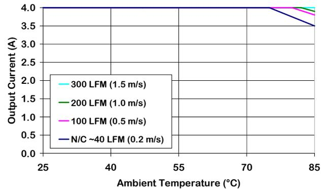
Figure 4. Output Current Derating vs Ambient Temperature & Airflow (converter mounted vertically with air flowing from pin 3 to pin 1, Vin = 24-36 V.)
