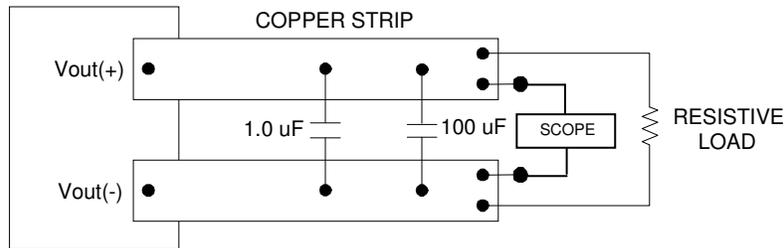
Use a 1.0 $\mu$ F X7R ceramic capacitor and 100 $\mu$ F X5R ceramic capacitor. Scope measurement made using a BNC socket. Position the load 3 in. [76mm] from module.
