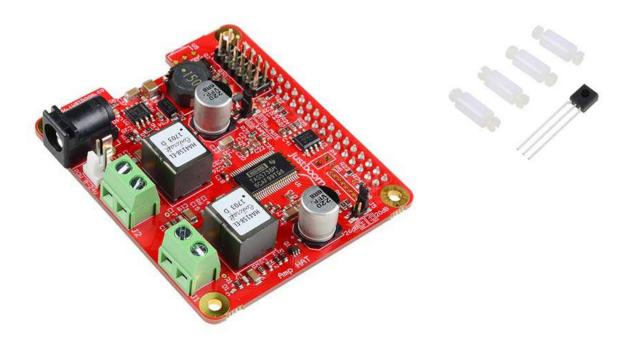
The JustBoom Amp HAT is a high-quality audio amplifier designed specifically for the Raspberry Pi. Digital-to-analog conversion is also included with the Amp HAT, so no external sound cards or DACs are required. Simply stack the plug-and-play add-on board (HAT) onto your Raspberry Pi A+, B+, 2B or the new 3B, and it will be ready to use immediately.
