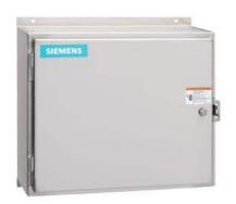
Mechanically held lighting contactor, Contactor amp rating 60Amp 0NC - 10NO poles, 208VAC 60HZ coil, Non-combination type, Enclosure NEMA type 12, Dust/drip proof for indoors
