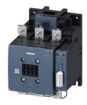
power contactor, AC-3e/AC-3 300 A, 160 kW / 400 V, AC (50-60 Hz) / DC Uc: 96-127 V PLC input 24 V DC 3-pole, auxiliary contacts 1 NO + 1 NC drive: electronic main circuit: busbar control and auxiliary circuit: screw terminal with remaining lifetime indicator
