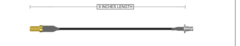
Connector A 132116RP SMA Jack Straight Brass Gold + Heatshrink 50 Ohm RG-58 Continuity/Hi-Pot Connector B 112202 BNC Jack Straight Bulkhead - Rear Mount Brass Nickel + Heatshrink
