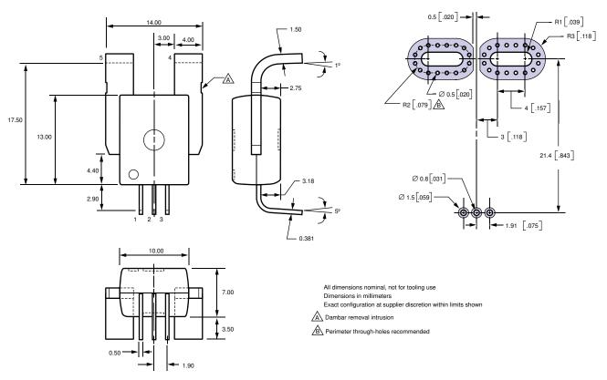
Creepage distance, current terminals to signal pins: 7.25 mm Clearance distance, current terminals to signal pins: 7.25 mm Package mass: 4.63 g typical
