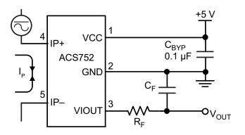
Application 1. The ACS752 outputs an analog signal,  $V_{OUT}$ . that varies linearly with the uni- or bi-directional AC or DC primary sampled current,  $I_P$ , within the range specified.  $C_F$ is recommended for noise management, with values that depend on the application.
