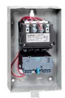
Non-reversing motor starter, Size 0, Three phase full voltage, Solid-state overload relay, OLR amp range 0.25-1A, Non-combination type, Enclosure type 12, Dust/drip proof for indoors, Standard width enclosure
