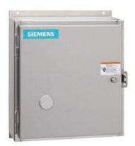
Mechanically held lighting contactor, Contactor amp rating 20Amp 0NC \_ 8NO poles, 208-240V 50/60HZ coil, Non-combination type, Encl NEMA type 4X 304 S-steel Water/dust tight noncorrosive
