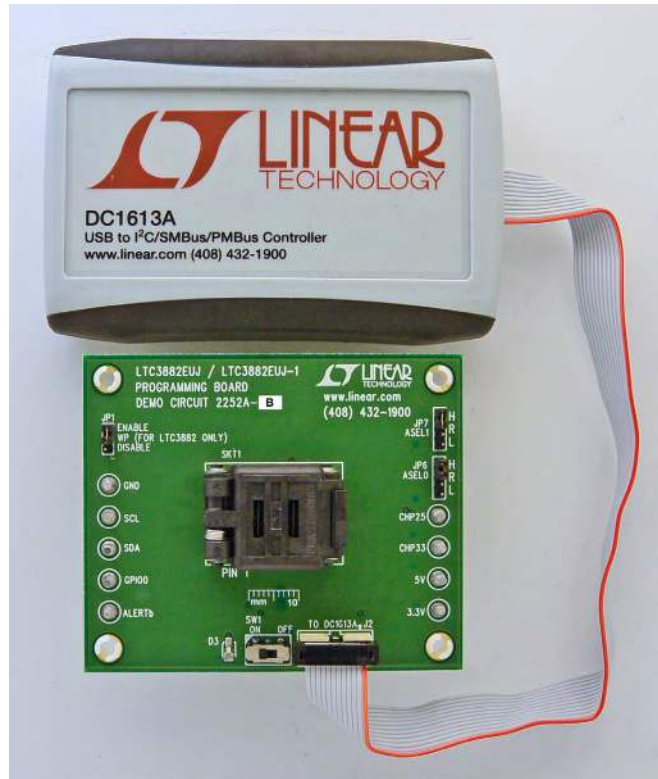
Figure 3. DC1613A Ribbon Cable Installation
