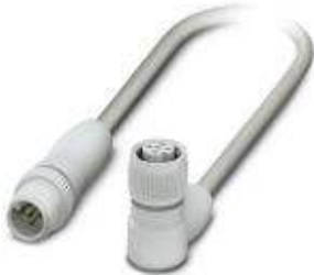
Sensor/Actuator cable, 5-position, PP-EPDM halogen-free, Gray RAL 7035, Plug straight M12, A-coded, on Socket angled M12, A-coded, Cable length: 1.5 m, Hygienic design, with plastic knurl
