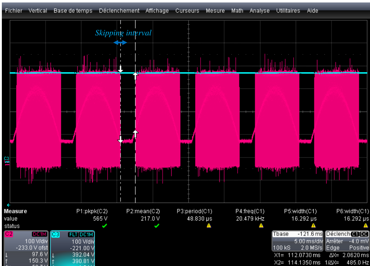
Figure 2 – MOSFET drain-source voltage ( V_{in,rms} = 230\text{ V}, I_{LOAD} = 0.1\text{ A} )
