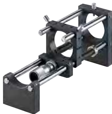
Example for a Z-translation with Holder for Micrometer, Micrometer G 10, Counter support, Compression springs and stop rings
