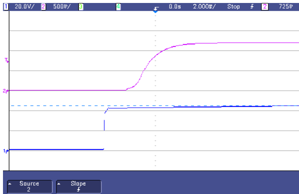
Fig.21 Typical start-up from power on of AGQ100-48S1V2
