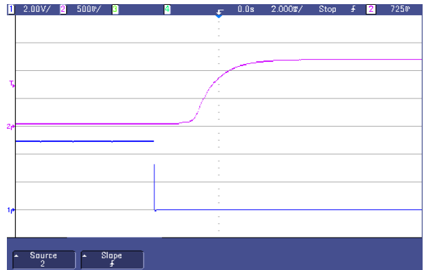
Fig.22 Typical start-up from CNT on of AGQ100-48S1V2
