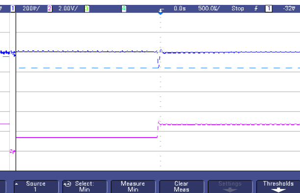
Fig.32 Typical transient response to step decrease in load from 50% to 25%, room temperature, 48Vdc input ( \Delta I_o/\Delta t = 1A/1\mu s ) of AGQ100-48S1V2
