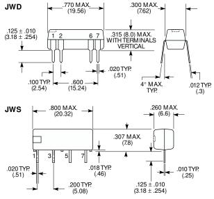
Note: Magnetic shielding may be required between relays when they are placed in very close proximity to one another.
