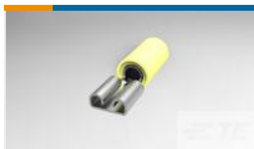
TE Part #8-640907-1 RECEPT,PIDG FASTON 12-10 250
