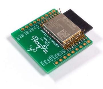
This board allows you to use various modules with a breadboard (and more) without having to solder the module in place. Just add FlexyPins.
