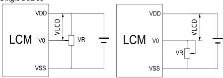
$V_{DD} \sim V_0$ : LCD Driving voltage
